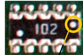
**SCALE: 1" = 1mm**    **NIC P/N: NRSN06C8 – Thick Film Chip Resistor Array**
