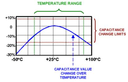
The maximum allowable change in capacitance value over a specified operating temperature range is the Temperature Coefficient (**TC**) of the capacitor
