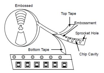
Remark: The sprocket holes are to the right as the tape is pulled toward the user.
