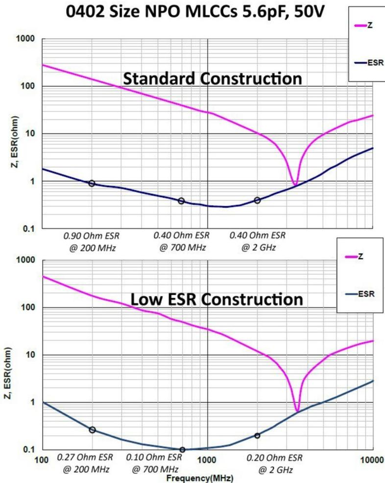
The table below shows the calculated 'Q' values based on the above ESR over frequency performance data.  $Q = X_c / ESR$
